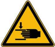
Warning, crushing hazard!
